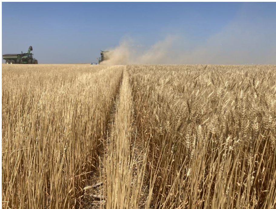
FIGURE 7: A FIELD OF WHEAT BEING HARVESTED WITH A STRIPPER HEADER IN SOUTH DAKOTA. SOURCE: AUTHOR'S OWN
